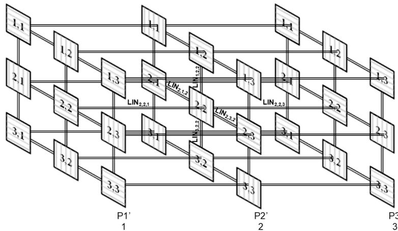
Fig. 4. Bidirectional communication lines between PCBs. Numbers indicate FPGAs (or ASICs) coordinates, while layers represent neighboring PCBs
