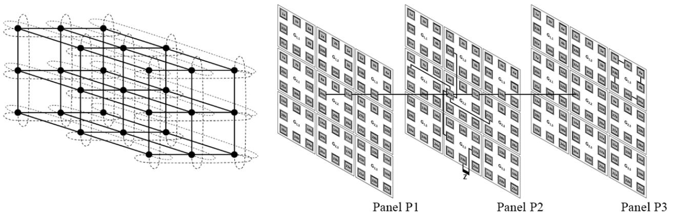
Fig. 5. Cell network with periodic boundary conditions (a) and system of connections between PCBs, which enables the system to be extended with periodic boundary conditions without a need to connect PCBs on the edge of the panels and on the outermost panels (b)
