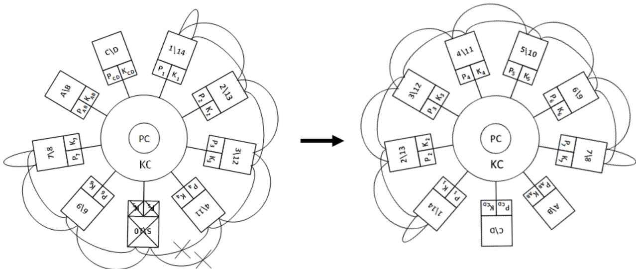
Fig. 7. Arrangement of panels in which 7 basic panels (1/14, 2/13, . . . , 7/8) and two additional panels (A/B) and (C/D) were used. This enables reconfiguration of the system in the event of a failure in one panel and/or signal lines connecting the pair of the other panels (a). Panels connections after the reconfiguration of the system as a result of failure of signal lines between the panels (4/11) and (5/10) (b)
